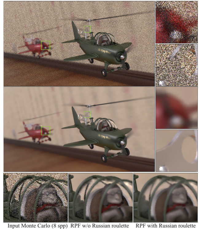
Fig. 13. Result of RPF on the TOY GYRO scene with 8D integration: DoF, motion blur, path-tracing, and Russian roulette for the cockpit window. The top image shows the MC input at 8 spp, the middle is produced by our algorithm. The bottom insets show that there is still noise after filtering if we do not include the Russian roulette term in the list of random parameters.
